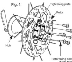
While wearing gloves, apply a force to the rotor to turn it in a clockwise direction as shown in Fig. 2. While doing this, tighten the rotor fixing bolts in the order shown in the illustration.
